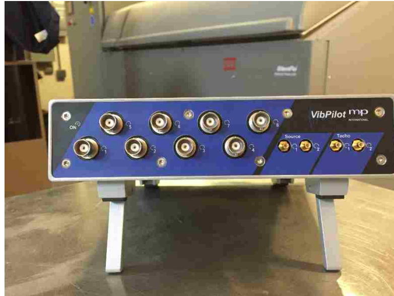
Fig. 3.6. Vibpilot Data Acquisition System.
