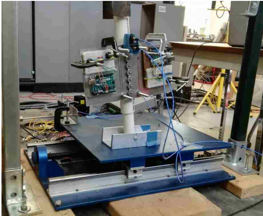
Fig. 5.3. Low-cost tilt measurement estimation set-up.
